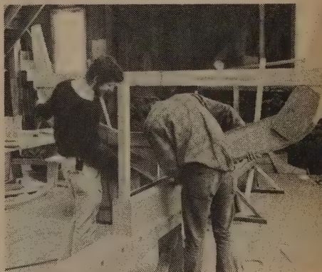
Setting up a mold on the keel assembly. The square holes in the sides of the keel are for the heels of the frames. Stefanie & Thomas Davies/Apprenticeshop .
